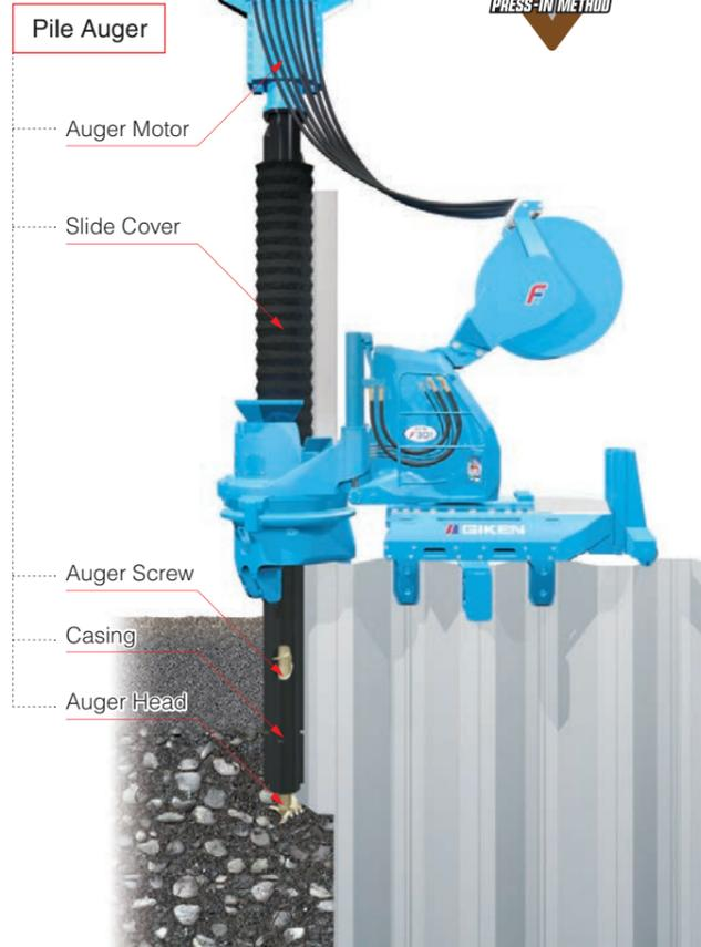
Crushing cobbles / boulders by wedge effect
