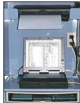
The Power Unit is connected to a PC and the state of press-in work is captured in real time.
