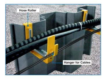
The Hose Roller prevents the hydraulic hoses and the power cable from damage. It also provides smooth working conditions for Silent Piler operations.
