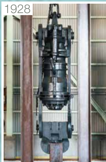
1928 Pile Extractor Reverse acting hammer for pile extraction
