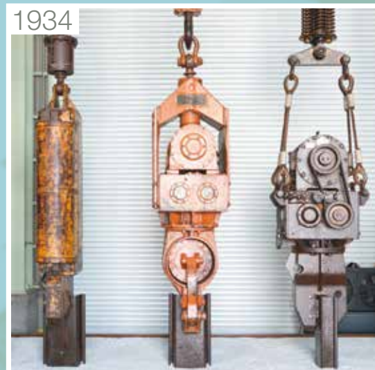
1934 Vibratory Hammer Vibration systems which drive piles using high frequency
