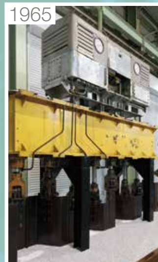
1965 Pile Master Multi-ram pressing machine with panel driving method
