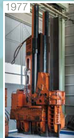
1977 KGK-100D First model of Silent Piler sold commercially
