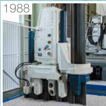
1988 TP333 First mass-produced Trench Sheet Piler
