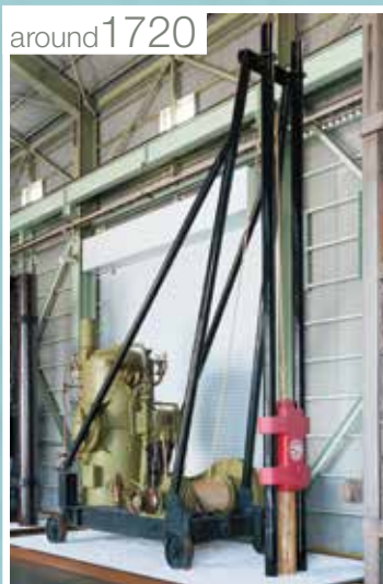
around 1720 Drop Hammer Pile Driver Drop hammer pile driver using steam power, among others
