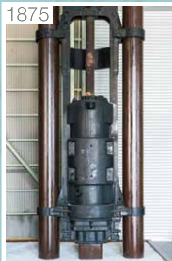
1875 Steam Hammer Impact driving systems with steam driven pistons
