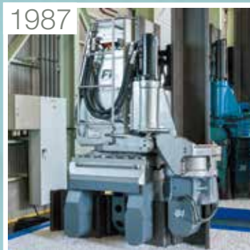
1987 FT70 Smaller, lighter, with full 360° rotation on Mast
