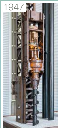
1947 Continuous Flight Auger (CFA) Machine that excavates and builds piles through augering
