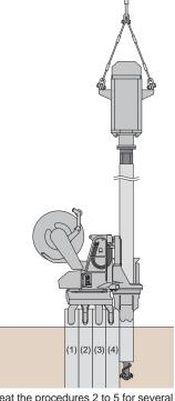
6. Repeat the procedures 2 to 5 for several sheet piles, then remove the Reaction Stand to complete initial piling.
