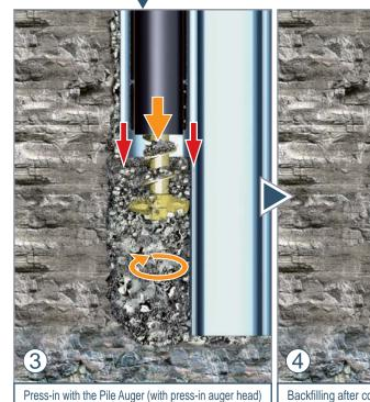
Replace the pre-auger head to the press-in auger head
