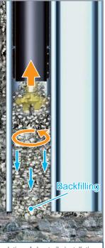
Backfilling after completion of sheet pile installation After completion of installation, while the Pile Auger is being extracted, the soil inside the Pile Auger are removed for backfilling.
