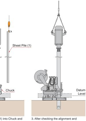
3. After checking the alignment and verticality, start pressing-in the sheet pile (1).
