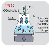
Activated sludge was used as microorganism source. Biochemical oxygen consumption (BOD) of specimen material (Piler Eco Oil & Piler Eco Grease 100mg/L) was continuously assayed by automatic assay system to valuate biodegradability (percentage of volume of
