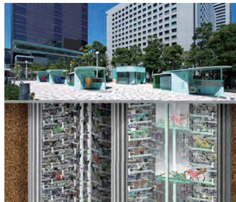
Earthquake-resistant underground bicycle parking GRIN Base (Minato-ku, Tokyo)
