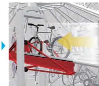
The carrier device fetches your bicycle.
