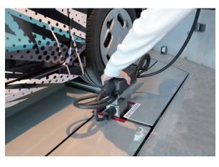
When parking the vehicle, you can easily charge it by performing a simple operation. The standard specification is 200V, but it can also be changed to 100V.
