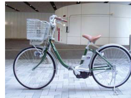
Electric assist bicycle compatible with automatic charging system
