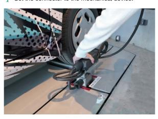
Connect the cable to the vehicle.
