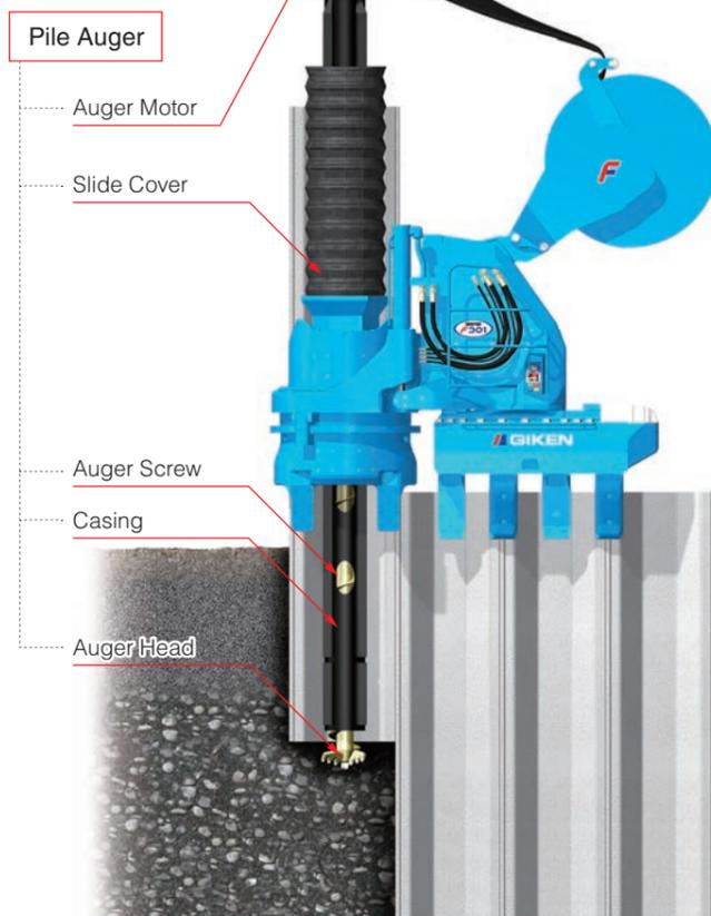
Crushing cobbles / boulders by wedge effect
